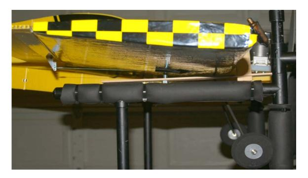
When balanced, the airplane will tip slightly nose down but not touching the surface below. (Note: Make sure the blocks do not interfere with the balance point; move them back from the LE if necessary)
