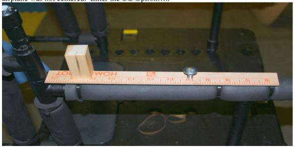
It is very simple ..... adjust the block to the desired CG position. The 4D calls for a 5" CG from the leading edge of the wing. . Set the airplane on the stove bolts with the leading edge barely touching the blocks.
