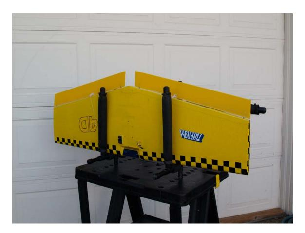
The Wing Thing is designed to hold the wing in either a horizontal or vertical plane. Mounted on the Stanley work bench, the wing is held a comfortable working level. You can rotate the bench 360 degrees to provide any angle of access you desire.
