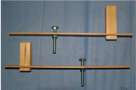
Assembled CG Parts ..... The nut below the ruler provides spacing for the bottom of the block. The height of the stove bolt can be adjusted to meet your specific application.
